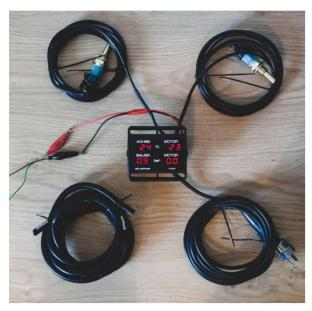
Your kit consists of the following parts: 1 control unit, 2 temperature sensors, 1 pressure sensor, 3 beams, 1 vacuum gas hose, 1 T for the hose, 1 metric adapter to install the sensor temperature on differential, various supplies ...
