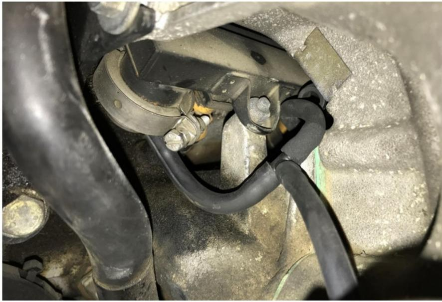
The intake gas pressure hose must be installed using the T-fitting on the hose leading to the fuel pressure regulator.
